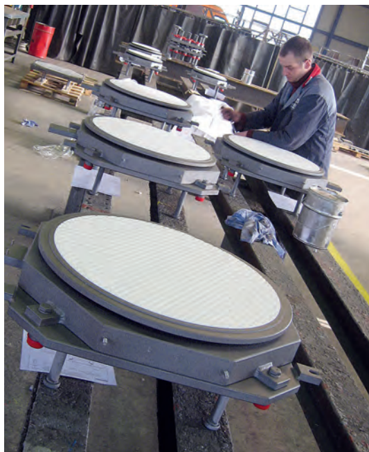
Assembly of free sliding pot bearings
