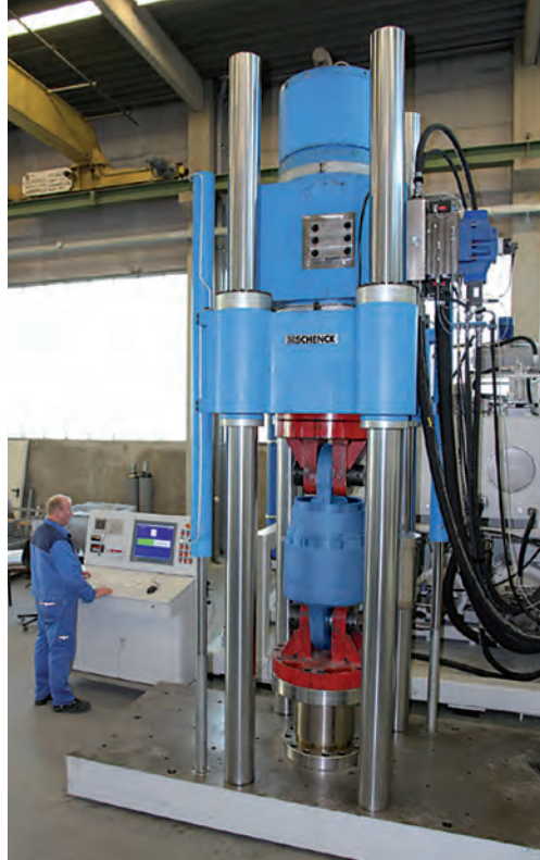
Dynamic test on viscous fluid damper at VICODA testing laboratory
